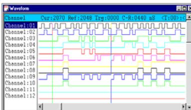
This screen shows up to 32 channels and lets you assign names to physical channel, rename signals and group signals into busses. The window also lets you zoom in on an area of interest. Markers and Cursors are provided to show the value at the specified time location.
