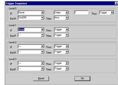
The sequence dialog box defines the sequence of occurrence of the trigger events defined in the Trigger Dialog box. Up to 4 levels of Trigger sequence can be programmed in an easy to understand **If...then... ButIf...** Format. A 64K event counter/ delay is also available for the first level of Trigger sequence.
